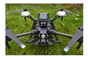
Use of several technologies embedded on the drone and the remote control's application to **automatically grab photos** at a good distance of the object and with a good overlap.
